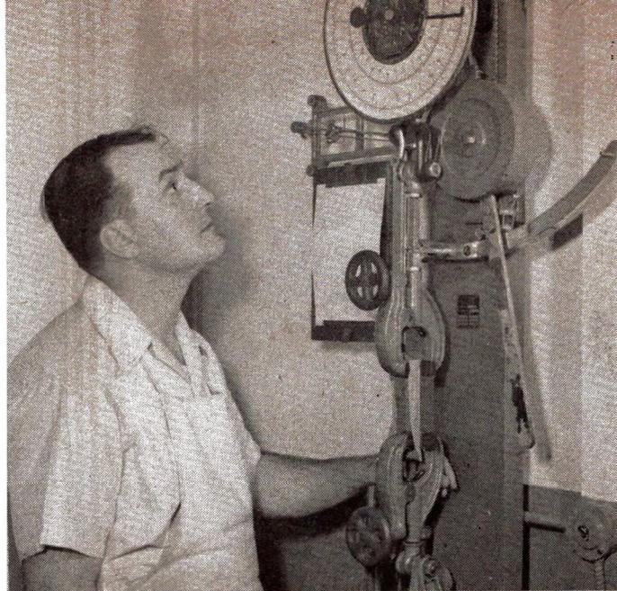
Samples of the material used in Marine uniforms are required to pass a high tensile strength test
